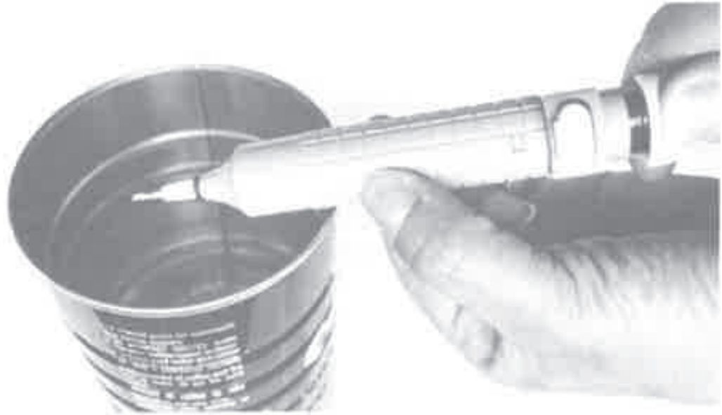
Figure 11-6 Discharge the waste solder into a can each time you recharge the tool. Otherwise, it just spits onto the keyboard.
