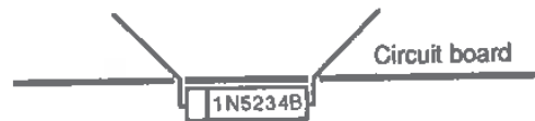
Figure 4-13 To prevent new parts from falling out when you lay the computer back down, pull up on the leads and bend them approximately 45 degrees.
