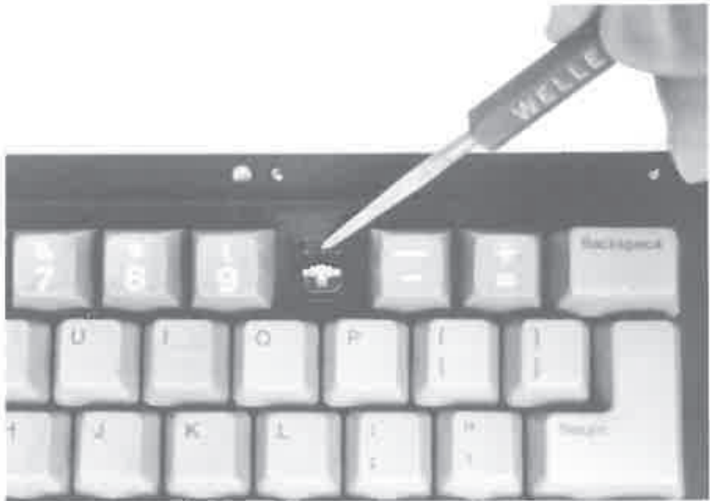
Figure 11-9 Depress one of the locking tabs with a soldering aid or a small screwdriver.
