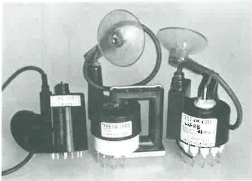
Figure 5-10 Flyback transformer types. The black transformer at the left came from an original 128K Mac. The gray and white transformer in the middle came from an early model Mac Plus. The solid gray transformer at the right is the latest, UL listed Macintosh SE type.
