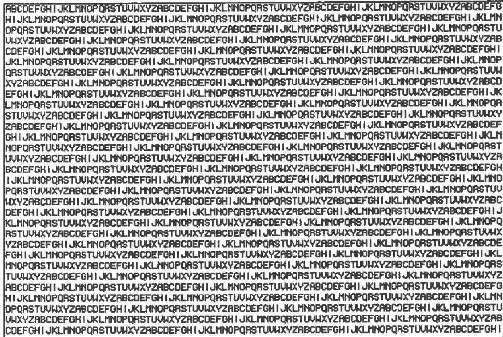
Figure 2-15 Focusing Text. Text at the corners should be just as sharp as the text in the center.
