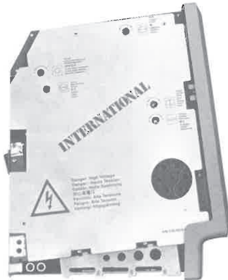
Figure 4-3 The 120/240-V board jacket is marked “INTERNATIONAL” in big red letters.
