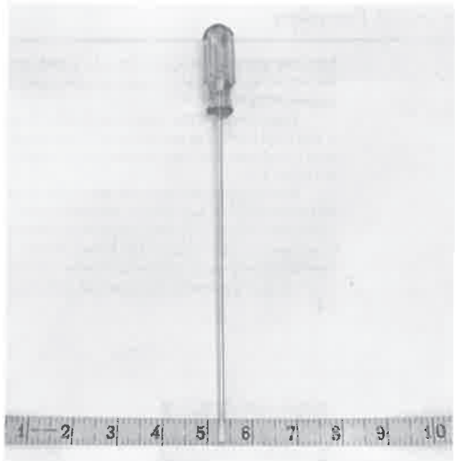
Figure 1-4 A precision ground flat-head screwdriver with an \frac{1}{8} -inch wide blade and an 8-inch long shaft.
