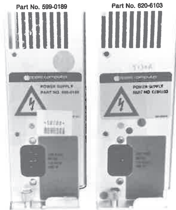
Figure 13-6 Lisa/Mac XL power supplies—external views. 1.8-A Lisa 2/10 to Mac XL power supply (left), and 1.2-A Lisa 2/5 power supply (right) are both marked “150W,” but the 1.8-A model is actually a dual voltage model, and it’s 50% stronger!
