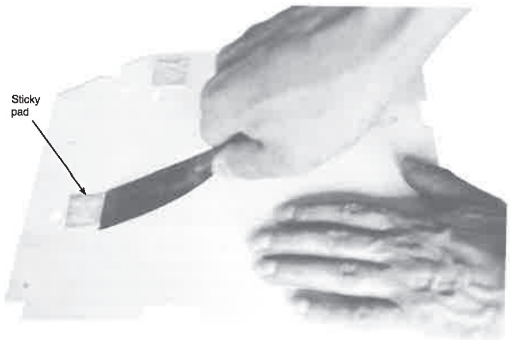
Figure 4-6 Cleaning the jacket. The easiest way to remove the old pads is with a putty knife.
