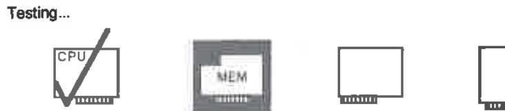
Figure 13-15 The Startup Module Test Display.
