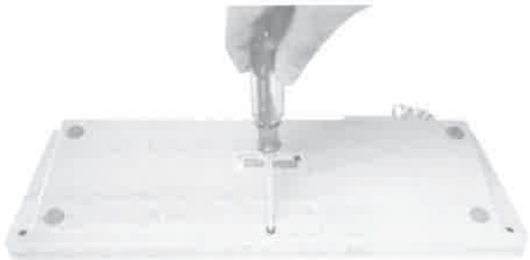
Figure 11-1 Loosen the screws in the bottom cover with a #1 Phillips-head screwdriver.
