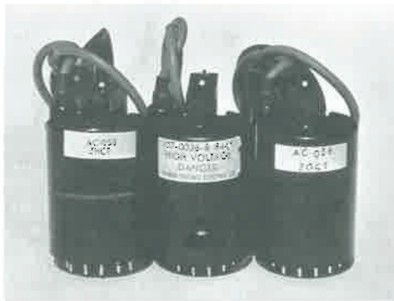
Figure 5-13 In advanced stages of failure, the case may show an obvious deformity.
