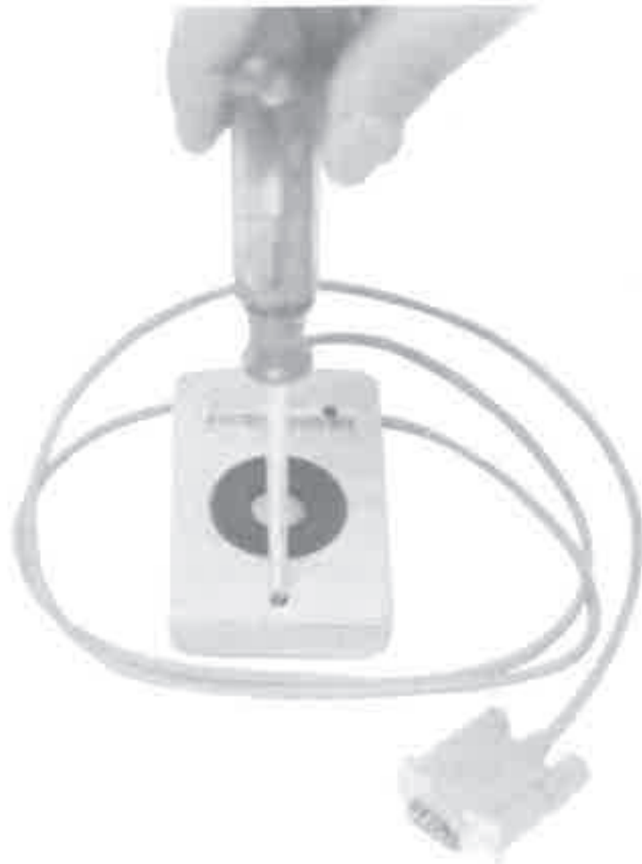
Figure 12-3 Loosen the screw or screws in the bottom cover with a #1 Phillips-head screwdriver.
