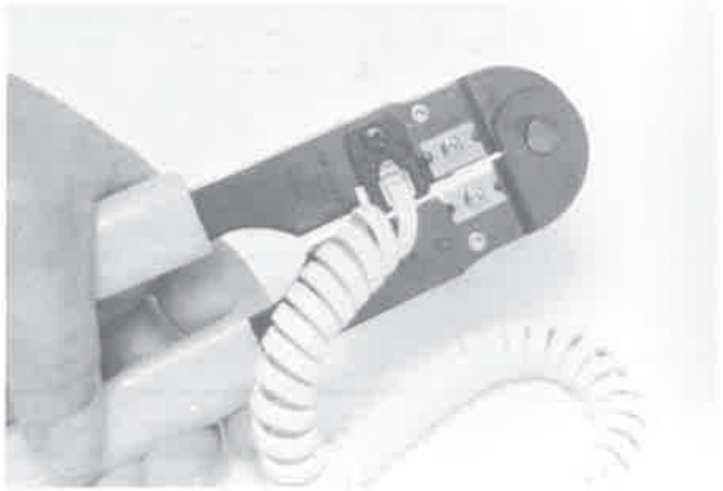
Figure 11-20 Crimping a new connector.
