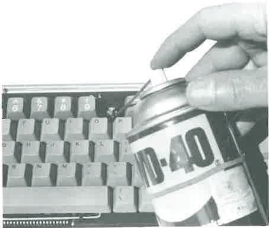
Figure 11-3 Intermittents can be treated with WD-40.
