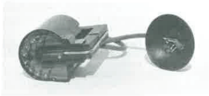
Figure 5-14 Usually there's evidence of burning on pin-4.
