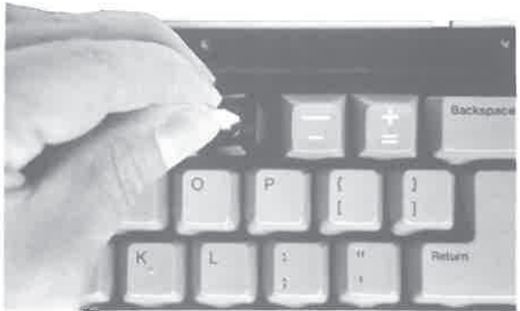
Figure 11-10 While pulling up on the key stem, try to release one side, then the other.
