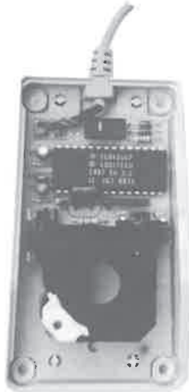
Figure 14-18 Inside the A9MO331 bus mouse.
