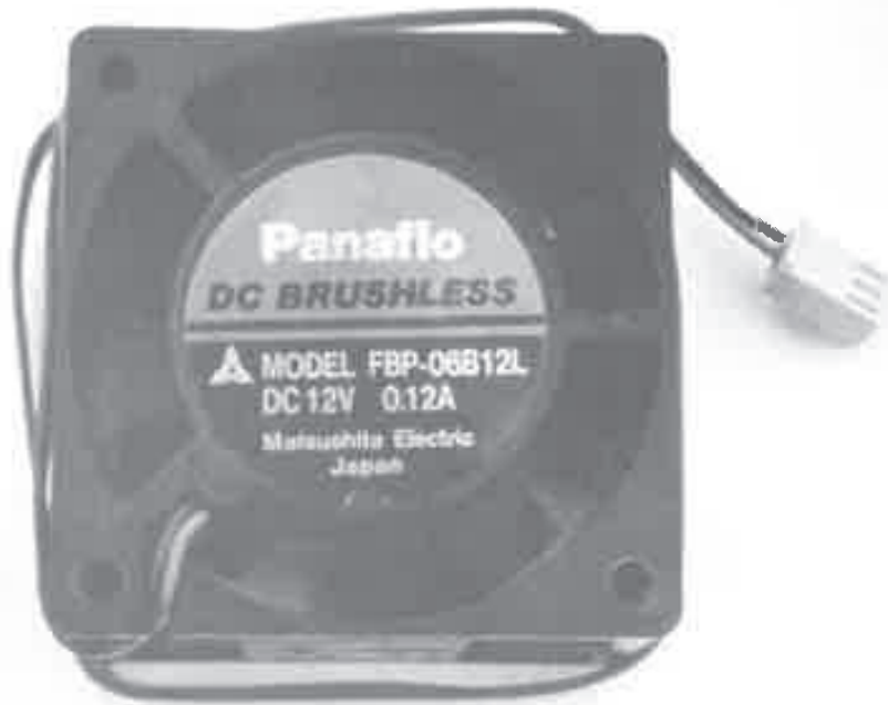
Figure 7-12 Boxer fan—128K to Mac Plus computers can be retrofitted with the same size fan supplied in the Macintosh SE.
