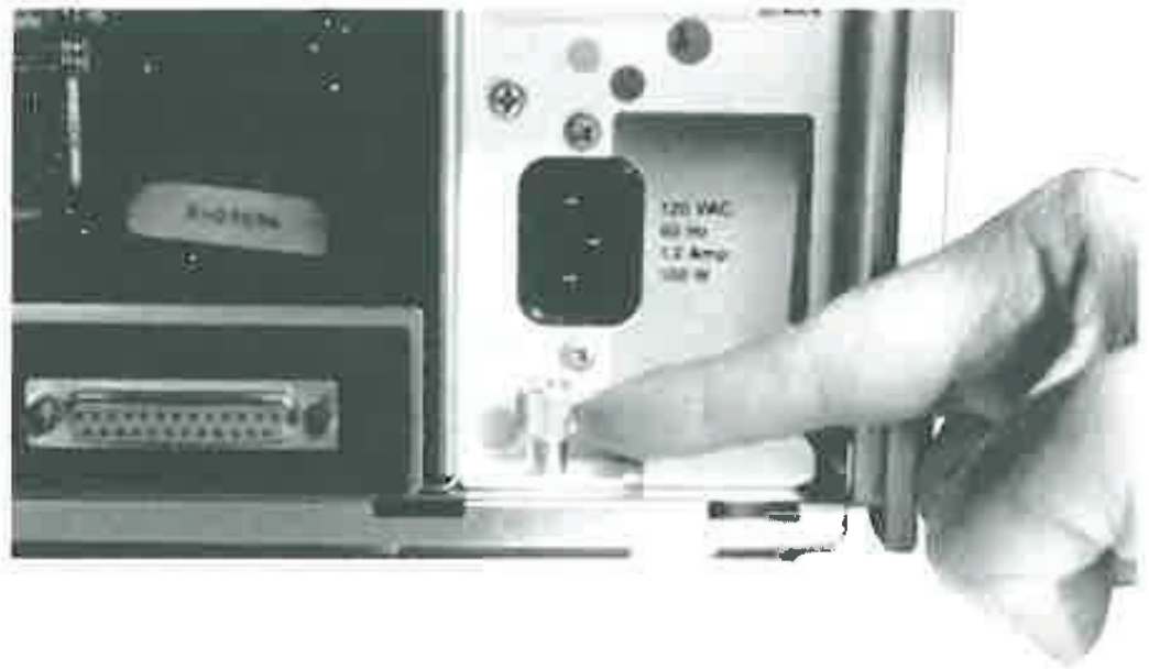
Figure 13-5 To remove the power supply, loosen the finger nut and pull straight back. Note that the nut is located approximately \frac{1}{2} inch from the edge of the chassis.
