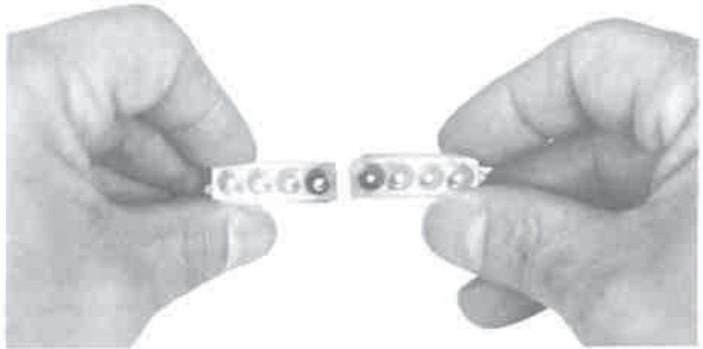
Figure 5-18 Burned J1 connectors. Note that the damage is always on pin-4, the horizontal sweep connection in series with C1.
