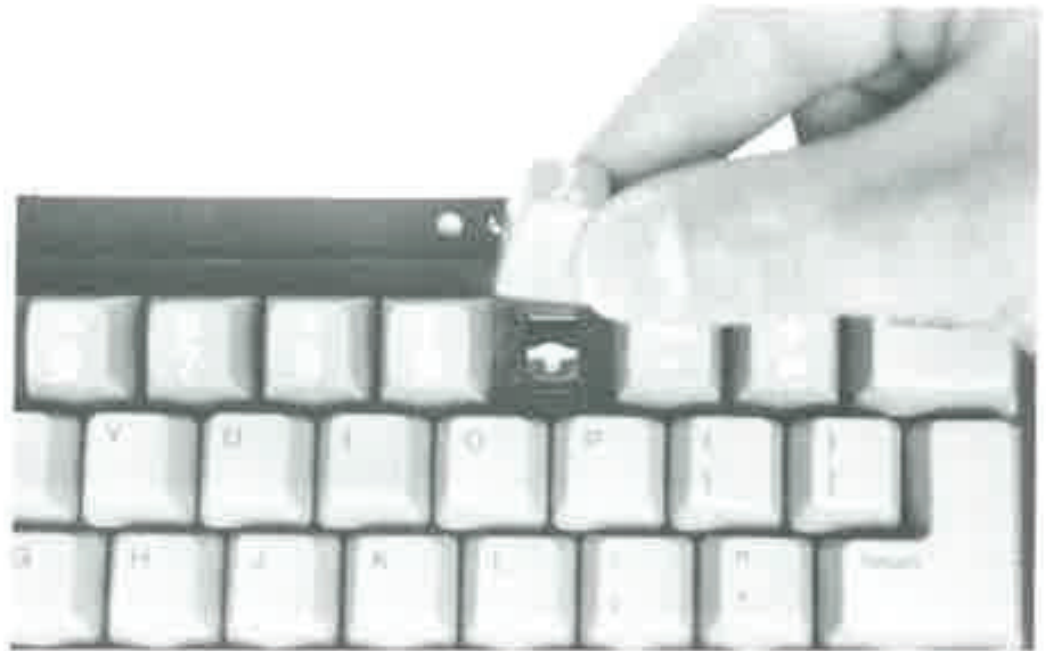
Figure 11-2 Remove the key cap by pulling straight up.
