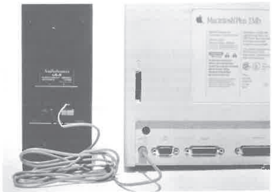
Figure 8-3 External speaker connections for the Macintosh Plus.
