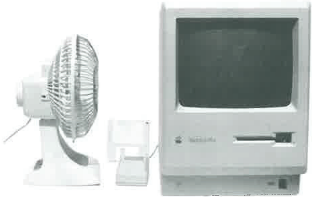
Figure 7-16 In dire emergencies, external oscillating fans may also be used.
